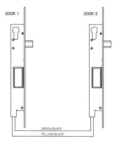
The electronic card housed in the lock allows to control two or more doors interlocked. Follow the above diagram: connect the yellow/black belt wire of the lock 1 to the same wire of the lock 2.
