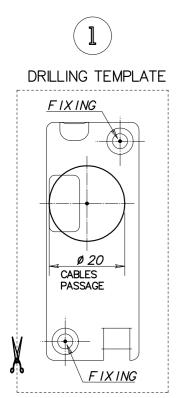
DRILL THE FIXING HOLES ON THE PROFILE AND THE Ø20 FOR THE CABLES PASSAGE. USE THE DRAWING AS DRILLING TEMPLATE
