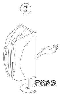
TURN THE ALLEN SCREW OF THE COVER IN THE ARROW DIRECTION UNTIL IT IS UNLOCKED
