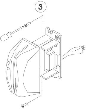
CONNECT THE CABLE TO THE CONNECTOR, THEN INSERT IT AND FIX THE BASE
