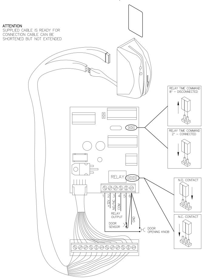
CONNECT A DOOR SENSOR/MICRO TO THE CIRCUIT, CLOSED ONCE THE DOOR IS CLOSED. READER IS ACTIVIATED ONLY WHEN THE SENSOR/MICRO IS CLOSED. IF THE SENSOR IS NOT INSTALLED, JUMPER 5 AND 6.
