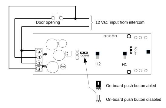
12 Vac connection with external transformer and opening command from intercom
